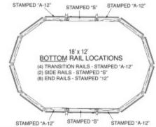
Place bottom rails stamped "S" between the side verticals. Place the bottom rails stamped "A-12" on the outside edge of the side supports as shown above. Place bottom rails stamped "12" on the ends of the pool.
