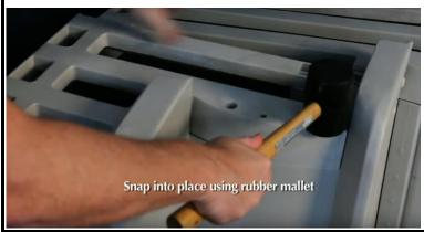
Step 11: Align ballast tray between all four risers under the step.
