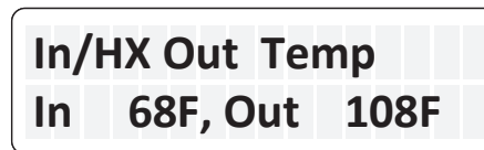
Figure 41. Inlet and Heat Exchanger Outlet Temperature
