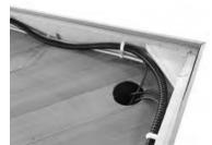
10. Feed the MAIN POWER CABLE through the hole in the ROOF and plug securely into the receptacle on the back of the POWER SUPPLY BOX. Secure the ROOF COVER with 3/4" SCREWS.
