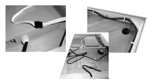
9. Feed the MAIN POWER CABLE through the hole in the ROOF and plug it securely into the receptacle on the back of the POWER SUPPLY BOX. Secure the ROOF COVER with 3/4" SCREWS.
