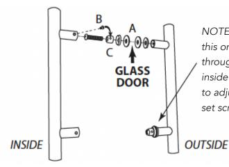
NOTE: The outside of the handle will look like this on the top and bottom, once it is assembled through the glass holes, and before attaching the inside handle using the set screws. You may need to adjust the fittings (C) so they line up with the set screw holes before inserting the screws.
