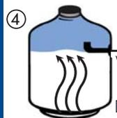
④ CLOSE FILTER AND BACKWASH UNTIL BACKWASH WATER IS CLEAR.
